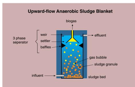
Figure 2. Flow-through Bio-reactors Using Granular/Immobilized Sludge: Upward-flow Anaerobic Sludge Blanket (UASB) Reactor.
