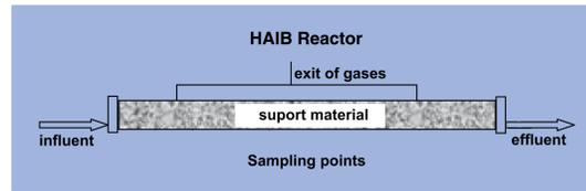
Figure 3. Flow-through Bio-reactors Using Granular/Immobilized Sludge: Horizontal Anaerobic Immobilized Bed (HAIB) Reactor.
