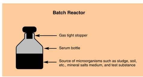
Figure 1. Batch (sealed vessel) bio-reactor for anaerobic biodegradation testing.
