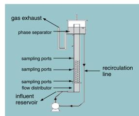
Figure 5. Expanded Granular Sludge Bed (EGSB) reactor
