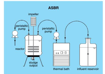
Figure 4. Anaerobic Sequencing Batch Reactor (ASBR).
