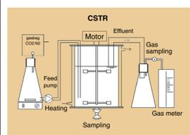
Figure 6. Continuous Stirred Tank Reactor (CSTR).
